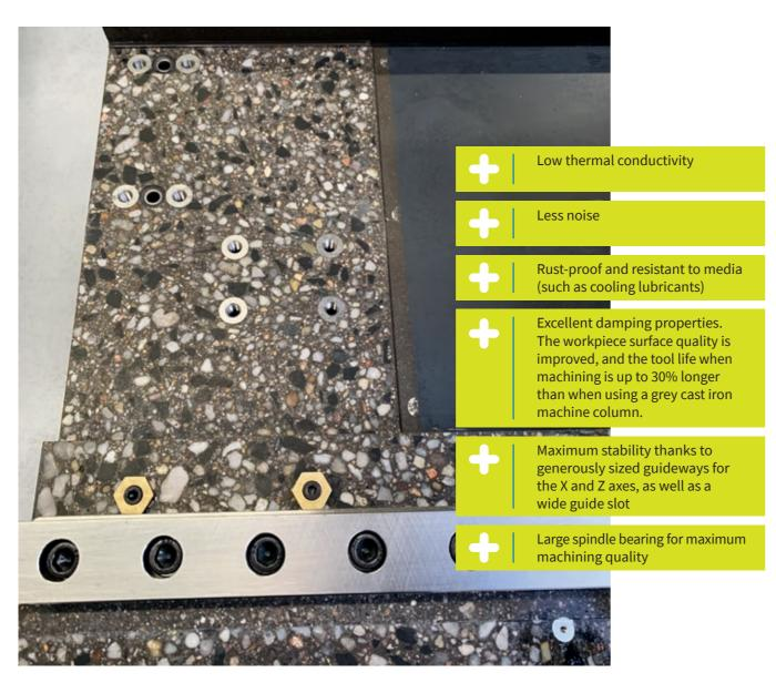
The machine column is the central element of the Schuster nxt. As in all machines from Schuster, the machine column of this pick-up lathe is made of cast Mineralit. It permits low-vibration machining for long tool life combined with uniformly high machining quality.
